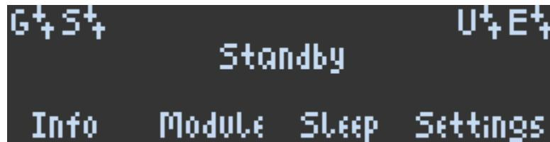
Indicators at the top of the screen show the status of connected interfaces: GPIB, RS232, USB and Ethernet. There is an up-down arrow to show active communications.
