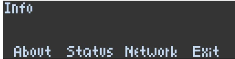
The first 'About' sub-screen shows information about the amplifier, manufacturer, model, serial number and firmware version.
